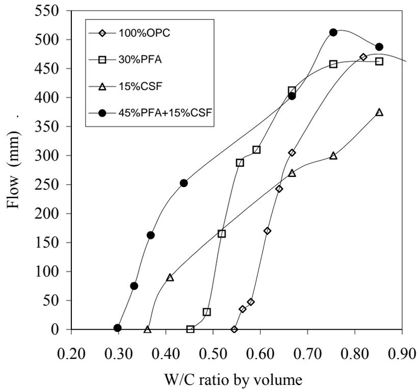
Figure 6 Flow value of cement paste at different mix proportions and water/cementitious ratios
