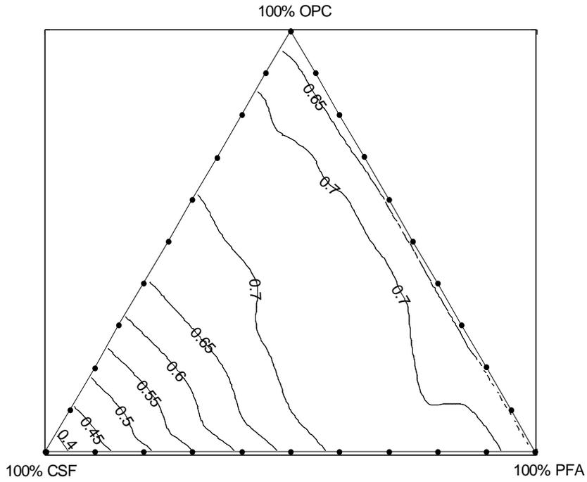
Figure 5 Contour showing the packing densities of cementitious materials at different mix proportions
