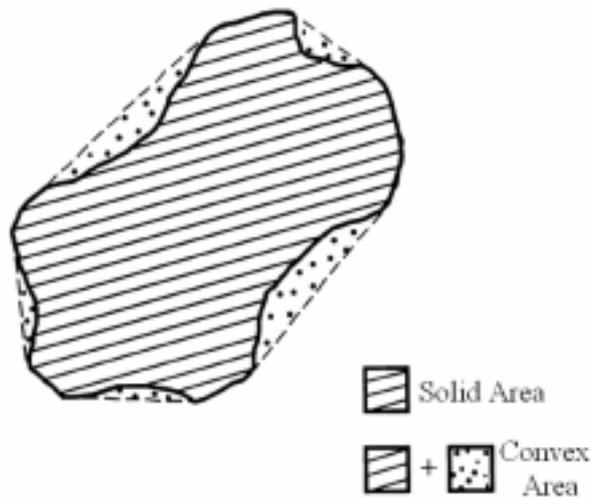
Figure 2 Definition of solid area and convex area (Kwan and Mora 2001)
