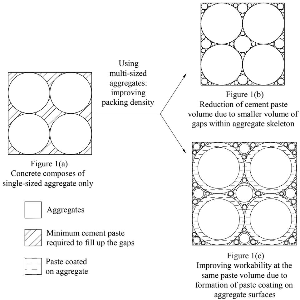
Figure 1 Packing of aggregates
